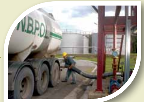
Transfer of oil from mill to land tanks at port of loading using dedicated tankers
